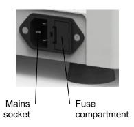
The following fuses are required for CENTRIC 260: 2 x 6.3AT 250V (230V) 2 x 10AT 250V (120V)
